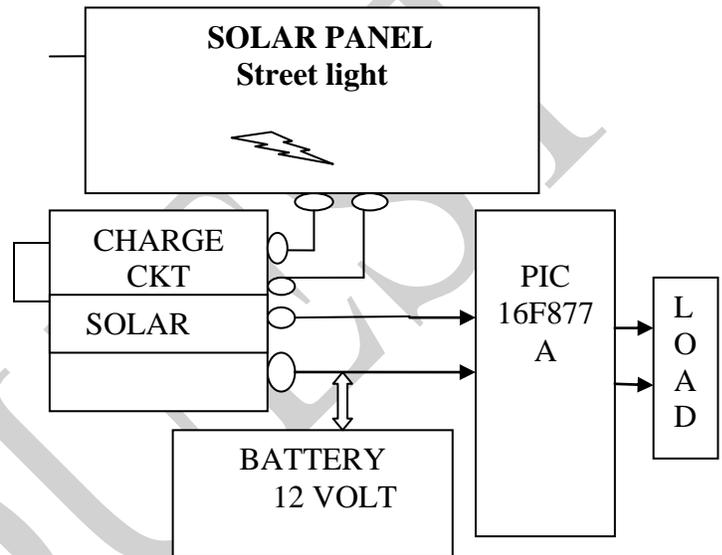
**Fig 3.0: Block Diagram of Solar Street Lamp**
