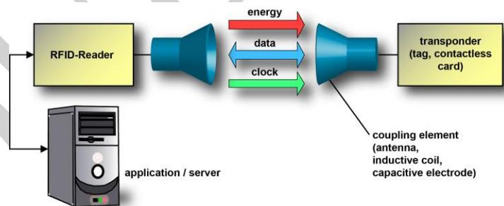
**Figure: 4** Radio Frequency Identification
